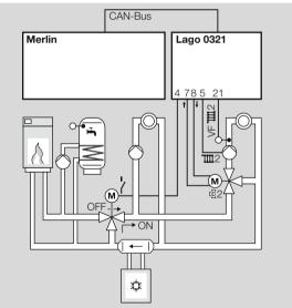
The central controller activates the "Cooling" operating mode via the CAN bus and controls the heat source, the refrigerating machine, the
