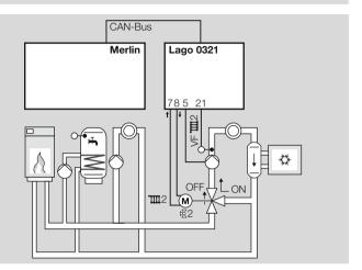
The mixer in the heating circuit functions as a valve. The mixer opens (ON). The heating circuit pump is switched on.
