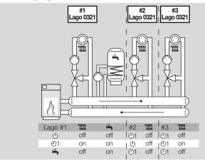
Lago#1 controls the first heating circuit and hot water. Lago #2 controls the second heating circuit and Lago #3 the third. If mode  $\circ$  was selected for Lago #1, the entire system will be switched off, regardless of the settings for the other controllers.
