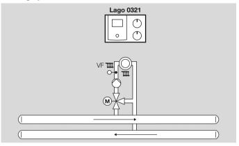
This application is automatically activated if only one flow sensor (VF/VFAS) is connected.
