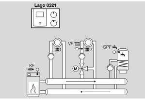
Connect heat source sensor (KF/KFS), flow sensor (VF/VFAS) and storage sensor (SPF/SPFS),
