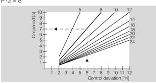
In the case of a controller deviation of 6 K the mixer is actuated for 7s and remains switched off for 3s.
